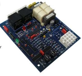
Analog Delay Determinator Circuit: Enerpro's gate delay determinator circuit is based on an analog PLL circuit and implemented with a proprietary ASIC. This circuit adjusts the gate delay firing angle in negative proportion to the SIG HI delay angle command signal.
